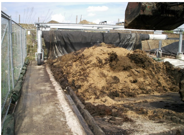
Foto 6: Refill: Fresh substrate is mixed with old substrate (inoculation).
